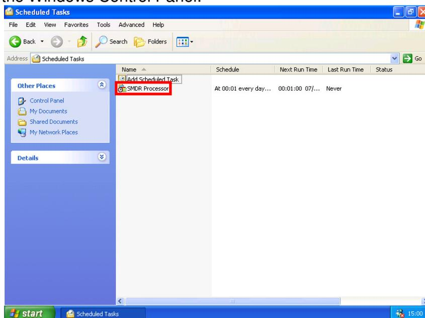
Right click the Processor task and select Properties. Un-tick the 'Enabled (scheduled task runs at specified time)' and click OK.
